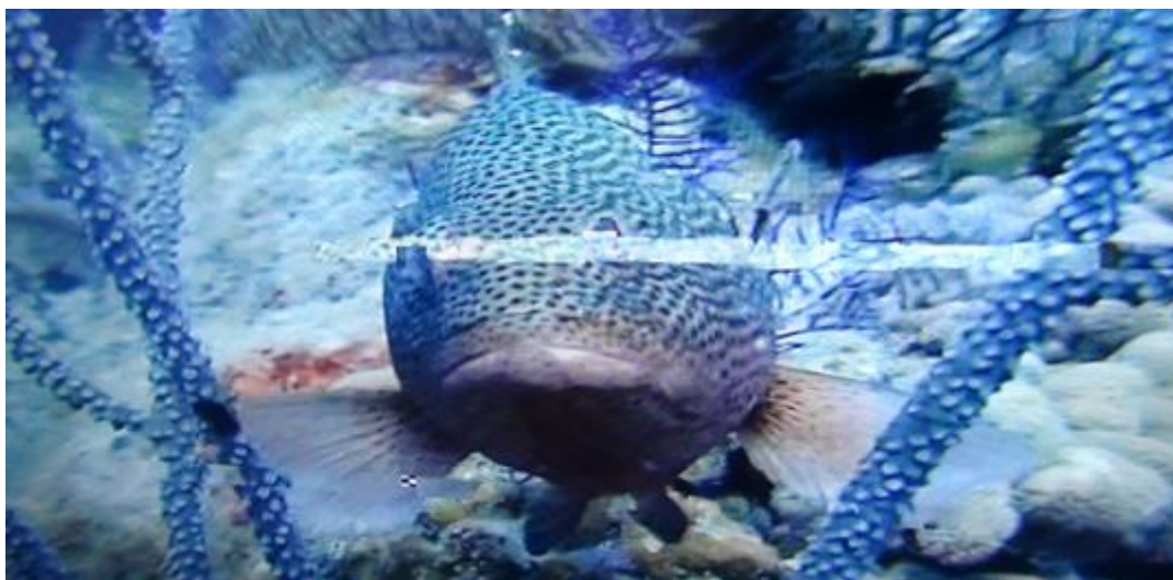
Figure 3 Example of picture failure caused by interference
